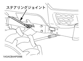
■ Inspection of the toe-in adjustment and the tie rod
